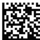
Datamatrix o GS1 Datamatrix
